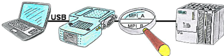
You're right in the middle of your production line and are standing in front of a passive assembly just like a switcher or a ET200, in that case you won't be able to go Online without an external power supply of your programming adapter, unless you're using the S7USB. This module is supplied completely from the USB-interface.
