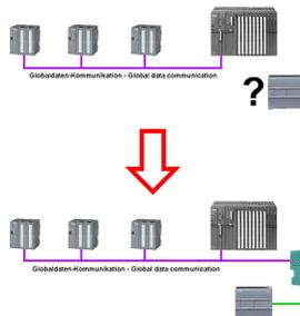
Running global-data-communication between MPI-PLCs (S7-300/400), is one of these PLCs replaced with a newer PLC with network-interface (S7-1200/1500), this PLC was not able to access this data.
