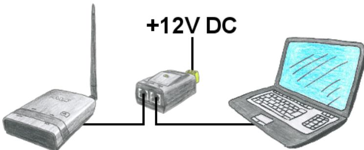
You dont want to power ALF with 24V DC because you have in your network PoE "Power over Ethernet" in use. No problem, ALS provides passive PoE, this means he can be powered with the not used cables of the lan-cable with 12V DC. You dont need additional the 24V DC.
