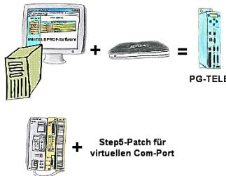
You're using the devices of the Tele-Network-family and don't want to have a device standing on the table? No problem. Install the WinTELEPROF-software on your PC and after link connection access to your Step5/7-programming software (also Siemens) via a virtual Com-Port.
