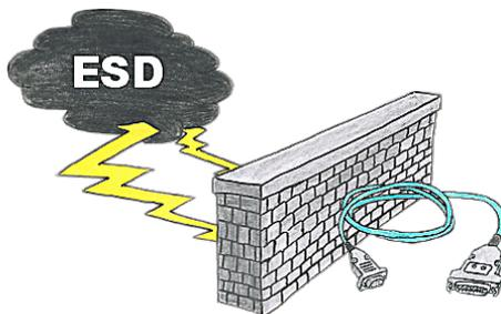
Safe communication with the S5-PLC in an environment of radiant-converters and motor-controls. Electrostatic-charging is also a KO-criterion for operation of interface-cable, a discharge and the interface-product is damaged or even defective.
