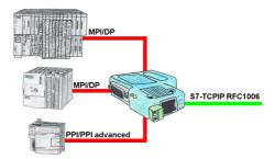
Networking of all S7-controllers (S7-200/300/400), for example with your production-data-acquisition, Industry 4.0 (OPC Server UA or Classic), panels and other devices that communicate via S7-TCPIP RFC1006. One module for all bus-types: PPI, MPI and Profibus.
