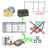
Via digital input triggered DB-backup/-restore without additional PC via PG-socket and Ethernet to FTP-server
