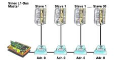
You have a running Sinec-L1-bus and your master the CP530 is defective or rather broke down and the bus has to continue running? No problem, connect the L1-controller to the according bus-modules instead of the CP530, define the circulation list of the clients and the L1-bus continues running immediately.
