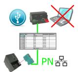
S7-PLC triggered DB-backup/-restore without additional PC via MPI/Profibus on USB-stick
