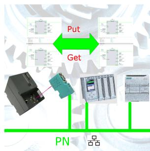
Coupling S7-controller with PN-port at S7-controller with MPI/Profibus via network
