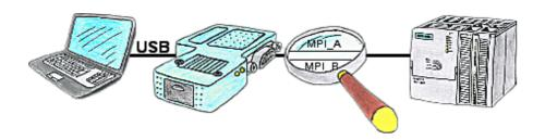
Your're right in the middle of your production line and are standing in front of a passive assembly just like a switcher or a ET200, in that case you won't be able to go Online without an external power supply of your programming adapter, unless you're using the S7USB. This module is supplied completely from the USB-interface.
