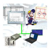
Replace defective panels in your "old" S5-systems with current and available S7-panels To do this, simply insert a placeholder PLC (e.g.  $315-2-PN\/DP$ ) in the WinCC-project, the IP-address of the PLC corresponds to the IP-address of the S5-LAN++-module. You can then visualize the data as usual.
