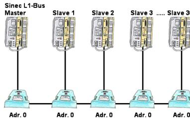
You have to configure a Sinec-L1-bus, own the master, but there's no BT-777-busterminal to buy? No problem, connect the IBX-Klemme to every S5-PLC that is in the run via the optional IBX-SPS-cable, supply every IBX-Klemme with ext. 24V DC if the PLC is not able to provide it, set-up the address 0 and define the actual L1-bus-address in the PLC. Now your master can communicate with the slave-assemblies.
