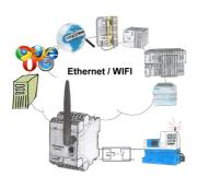
Switch with the EtherSens Control with relay-output easily and directly over LAN or WIFI up to 230VAC/16A, switchable over web-browser, TCP/IP-protocol or PLC-controlled. At the same time you monitor the switching-states on the optional SD-card or on the FTP server.
