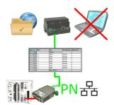
S5-PLC triggered DB-backup/-restore without additional PC via PG-socket and Ethernet on FTP-server
