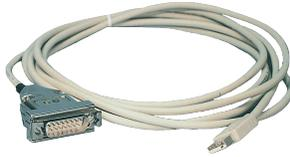
The PG-USB-Kabel is an interface cable for the 15pin PG-Port X4/X5 of a S5 plc. The cable should be connected to the USB-Port (type A-connector). This cable will be active against the plc while the power will be taken from the usb-port of the PC. For some special slot cards for the S5 you can get some special adapters with the several pinning of this card.
