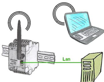
Access parallel via LAN and Wifi to the EtherSens-device. Therefore create via the web-server for each way an ip-address, regardless whether its the same subnet or not.
