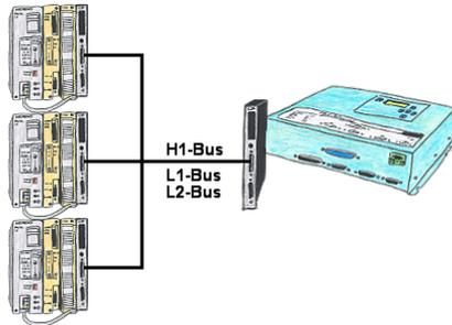
You have an existing L1-, L2- or H1-bus on the customer side and have to program parallel the PLCs? No problem, just connect the communication processor (CP) with a monkey swing to the PLC, the Tele-Network-device with the TELE-CP-cable to a free CP and select the needed PLC with PG-path selection. Therefore the L1-, L2- or H1-option is needed.
