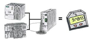
You need an exact time for your S7-plc? No problem, the TeleService-GSM fetches the current time via GPRS from a time-server and advises it to the S7-plc. How often and whenever the time shall be updated can be parameterised in the device.
