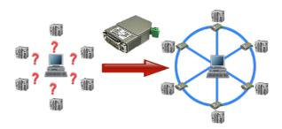
Your machines are fully distributed in your company area, it is not always a PC connected with the machine. What could be better than to connect the machines to your company network and backup the data central from one point!
