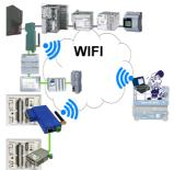
Wired or wireless communication (WIFI) via the same adapter with the respective control Devices from the BRIDGE-family always connect a wired-network with a wireless-network (WIFI) and a specific PLC-interface. This gives you access to the directly connected controller via WIFI (with S7 to the entired bus) as well as to the wired Ethernet. Of course also from wired Ethernet to WIFI and control/bus.
