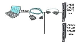
You have a PC with programming software and a 9pin COM-port as interface? No problem, for this purpose the PG-UNI-cable is exactly the right product. Connect it to a Siemens assembly such as H1-CP (CP1430), WF470 and PC or CP-525 with the CP525-adapter and PC and you're Online.
