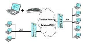
The Tele-Prof-II can also be used as a router for access from a PC via dial-up connection, so that a communication with the behind covered network results. Furthermore a network connection can be made with the TP-II TP-II-line, but in doing so the IP-address-root must differ.
