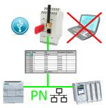
S7-PLC triggered DB-backup/-restore without additional PC via PN-port to USB-stick
