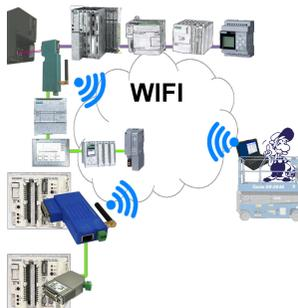
Wired or wireless communication (WIFI) via the same adapter with the respective control Devices from the BRIDGE-family always connect a wired-network with a wireless-network (WIFI) and a specific PLC-interface. This gives you access to the directly connected controller via WIFI (with S7 to the entire bus) as well as to the wired Ethernet. Of course also from wired Ethernet to WIFI and control/bus.
