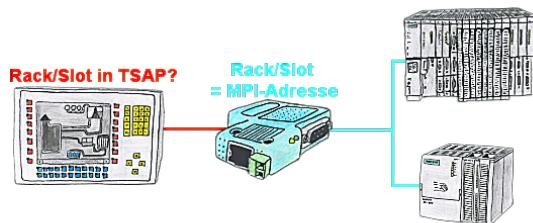
Your panel or visualisationsystem addresses the used PLC with Rack/Slot in TSAP? No problem, activate this mode in the S7-LAN and you will get actual data from the PLC.
