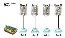
You have a running Sinec-L1-bus and your master the CP530 is defective or rather broke down and the bus has to continue running? No problem, connect the L1-controller to the according bus-modules instead of the CP530, define the circulation list of the clients and the L1-bus continues running immediately.
