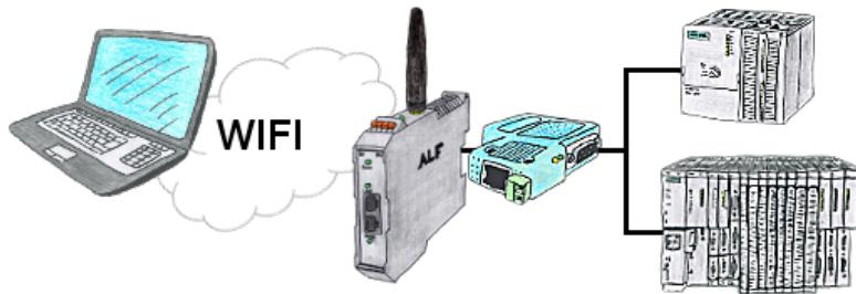
You're right in the middle of your production line and should move around the machine and simultaneously observe / manage. No problem, you parameterize the ALF, connect to the S7-LAN and connect to the WIFI-network of the ALF and are ONLINE on the PLC.
