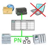
S7-PLC triggered DB-backup/-restore without additional PC via PN-port on FTP-server
