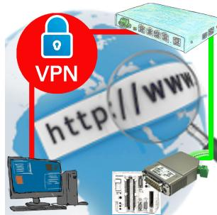
Remote-maintenance of a Siemens-S5-controller with S5-LAN++ on PD-port via secure VPN-tunnel of the TeleRouter
