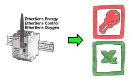
Capture the required values, whether if energy-data, states of inputs or outputs, process values such as oxygen-content in the environment,... and write this with a timestamp in a CSV-file. This file can then be read and processed with Excel.
