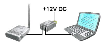
You dont want to power ALF with 24V DC because you have in your network PoE "Power over Ethernet" in use. No problem, ALS provides passive PoE, this means he can be powered with the not used cables of the lan-cable with 12V DC. You dont need additional the 24V DC.
