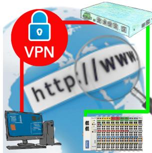
Remote-maintenance of a Beckhoff-controller with network-connection via secure VPN-tunnel of the TeleRouter
