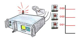
You need some limits? No problem, with the OSC-II-devices you will be able to define 3 relay outputs (toggle switch) like UG (down level) or OG (top level) or as a ready-flag (internal probe has working temperature).
