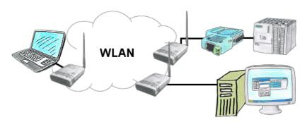
You have two or more clients which should communicate together without LAN-cable-connection? No problem, you connect a "Access-Point" configured ALF to this device and to the other device a "Client" configured ALF. Then connect the "Client" with the "Access-Point" and the device are able to communicate together.
