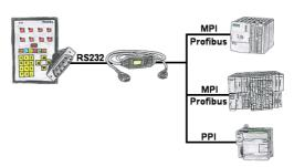
Your panel provides a serial port and no MPI/Profibus for connecting a S7-PLC. Connect the MPI/PPI-cable with it and you're Online with your panel.
