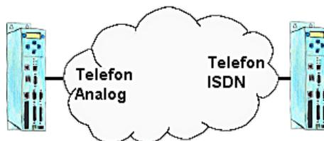
You have on the plant side only ISDN for telephone, but in your office there is only an analogue system? No problem, you have to install on the clients side the TP-II and activate there the analogue-emulation in the device. No, the modem signals will be sent digitalized over ISDN and you can connect to it. So, you will be able to communicate though the telephone systems are different and your client isn't forced to install an analogue connection.
