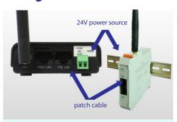
1 Connect the 24V power source and the computer to configure
