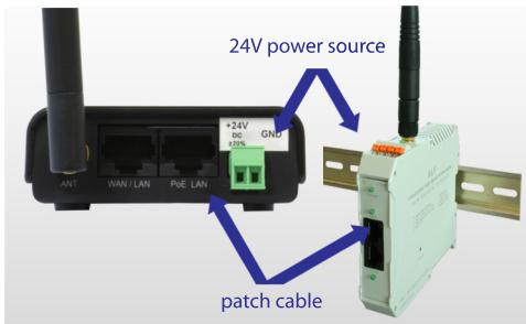
**1** Connect the 24V power source and the computer to configure
