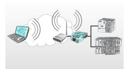
Connect the S7-LAN with a patch cable
