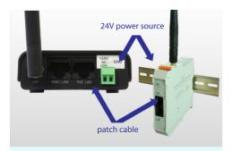
1 Connect the 24V power source and the computer to configure
