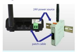
1 Connect the 24V power source and the computer to configure
