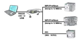
PLC-programming/-communication from the PC "serial" or via "USB" from S7-200/300/400 or modules such as Sinamix, Sinumerik, MicroMaster, drives, converters. PPI up to 187.5 Kbit (PPI + PPI advanced), MPI/Profibus up to 12 Mbit. Compatible with the Siemens driver "PC-adapter", communication only with 64-bit operating-systems via USB and TIC-driver (limitation of serial communication from Siemens to 32-bit operating-systems).
