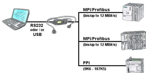
PLC-programming/-communication from the PC "serial" or via "USB" from S7-200/300/400 or modules such as Sinamix, Sinumerik, MicroMaster, drives, converters.
