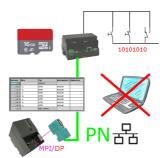
Via digital input triggered DB-backup/-restore without additional PC via MPI/Profibus to SD-card
