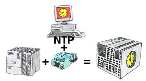
You need in your PLC a actual time? No problem, with the NTP-function the S7-LAN-module get from a NTP-(Time-)Server the actual time and transfers it direct into the configured PLC or for processing in a DB.
