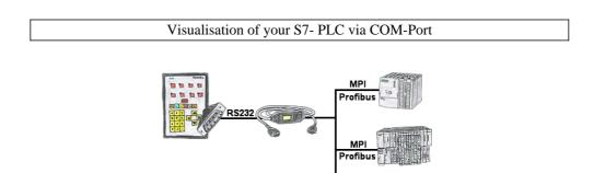
Your panel provides a serial port and no MPI/Profibus for connecting a S7-PLC. Connect the MPI/PPI-cable with it and you're Online with your panel.
