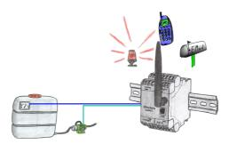
Apply small control tasks of your systems with EtherSens-Control-devices. Determine switching points where the device is running to respond. Depending on the parameterization, an email or SMS notification (depending on the device-configuration) or the device automatically controls via the optional IO-modules (analog / digital / relay).
