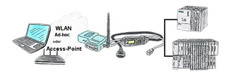
Your're right in the middle of your production line and and should move around the machine and simultaneously observe / manage. No problem, you parameterize the S7-WLAN-Bridge, connect to the MPI-LAN and connect to an access-point or with the ad-hoc-network of your laptop and are ONLINE on the PLC.
