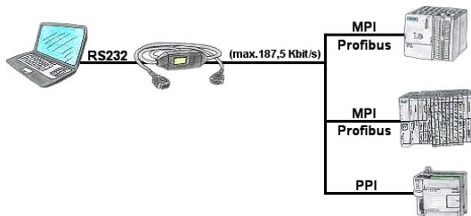
With the MPI/PPI-cable you have the ability to access a connected SPC-PLC S7-200 (PPI 9600 Baud and 19200 Baud) as well as S7-300/400 (MPI/Profbus 9600 Baud up to 187500 Baud) via PC serial with up to 115200 Baud for reading respectively writing of data.
