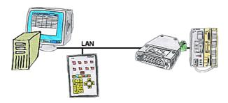
Your panel only has a LAN-socket as PLC-interface, no problem. Connect this socket with the S5-LAN++ and plug it directly on the PD-interface of the PLC. Then access to the variables and data of the PLC is already available.
