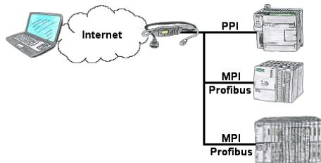
You have access to a on-site network and your PLC-device has no LAN-connection? No problem, plug the S7-LAN on the PLC-device and you will have immediate access to the PLC from afar.
