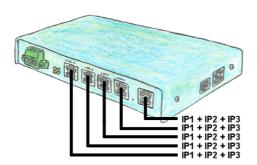
You need to remote maintenance multiple networks simultaneously and your existing switch / router does not have that many ports? No problem, with the TELE-Router you are able to assign up to 3 IP addresses to each LAN / WAN port, so you can communicate with the various segments and networks.
