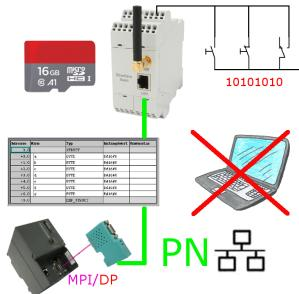
Via digital input triggered DB-backup/-restore without additional PC via MPI/Profibus to SD-card
