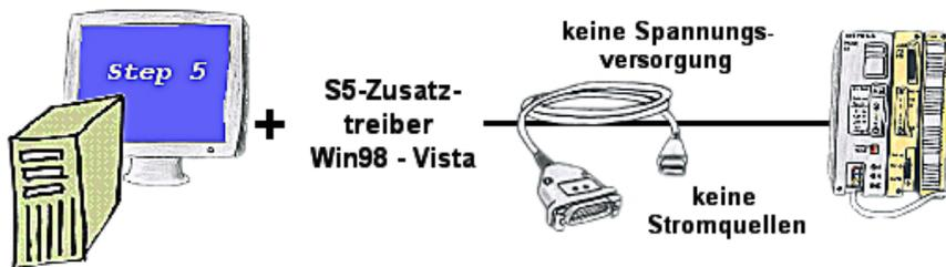
You still have a PC with Win98 and Step5-package and would like to go Online on your S5-PLC via USB? No problem, the provided virtual Com-Port PLCVCom emulates a COM-port on your PC with which you go Online. With a patchtool for the Siemens Step5-software, which is provided as well, nothing else stands in your way to communicate via LAN.
