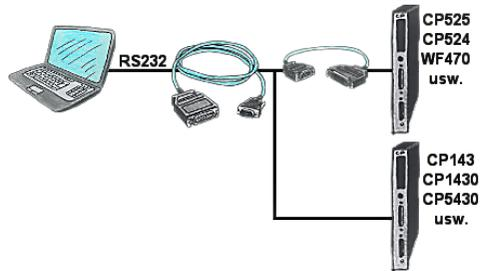
You have a PC with programming software and a 9pin COM-port as interface? No problem, for this purpose the PG-UNI-cable is exactly the right product. Connect it to a Siemens assembly such as H1-CP (CP1430), WF470 and PC or CP-525 with the CP525-adapter and PC and you're Online.
