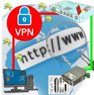
Remote-maintenance of a Siemens-S5-controller with S5-LAN++ on PD-port via secure VPN-tunnel and scalable firewall
