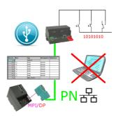
Via digital input triggered DB-backup/-restore without additional PC via MPI/Profibus to USB-stick
