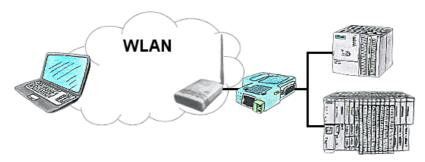
You are on site your plant and should move round the machine and simultaneously control or monitor. No problem, you parametrize ALF as an access-point and connect your S7-LAN or other network-client to him, connect your PC with him and you are online on the PLC.
