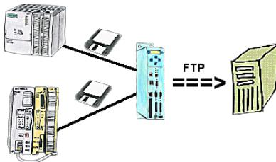
You need a data logger which tape-records the specified data of the PLC and you can collect the data via FTP on demand. No problem, TP-II with the option Datalogger is the solution for you.
