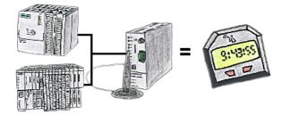
You need an exact time for your S7-plc? No problem, the TeleService-GSM fetches the current time via GPRS from a time-server and advises it to the S7-plc. How often and whenever the time shall be updated can be parameterised in the device.
