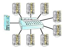
You have many PLC and you want to programm them central on one place? No problem, you have to connect them all to the KOR/MUX-Tele-Switch, connect it with the TP-II and after telephone connect you will be able with the PD-bus-selection of your Step5-software to go ONLINE. Of course the MOR/MUX-Tele-Switch is cascadable, so you can connect up to 30 PLCs to the devices.
