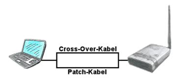
You need ALF to connect to a reachable WLAN, but only have a patch-cable? No problem, ALF provides "autonegotiation" and this means that he recognises a connected cable (patch-cable or cross-over-cable) and surround the pinning according to the cable, so a communication is possible.
