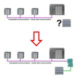
Running global-data-communication between MPI-PLCs (S7-300/400), is one of these PLCs replaced with a newer PLC with network-interface (S7-1200/1500), this PLC was not able to access this data.
