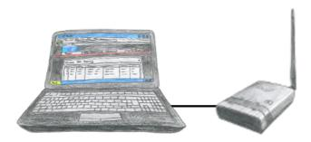
To configure ALF you dont need additional driver or special cables, you connect your PC via LAN or WLAN with ALF and over the integrated webserver you can configure the needed function.
