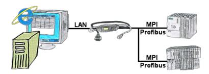
You would like to give your customer the opportunity to read current numbers of the manufacturing Online, without installing a visualisation or even the STEP7-package? Then a S7-LAN with the option Status Variable" is needed, and your customer can take a look at these password protected data on a site of the integrated webserver.
