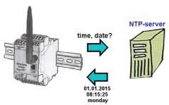
Should all EtherSens devices record time-synchronized in your equipment? By coupling with an NTP-time-server, all devices pick up the current time and adjust this.
