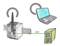
Access parallel via LAN and Wifi to the EtherSens-device. Therefor create via the web-server for each way an ip-address, regardless whether its the same subnet or not.
