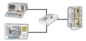
Your PD-interface of the S5-PLC is already occupied with a panel and you should accomplish program modifications without removing the panel? No problem, connect the Multiplexer one-time to the PLC and then connect the panel and also your PC to the Multiplexer. Now you can work parallel with the PLC without the need of affecting the operation of the panel.
