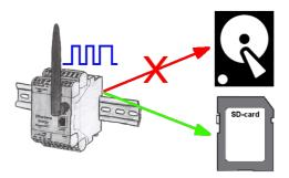
With the integrated SD-card-slot you back-up the recorded data in the device and dont need an external memory. Nevertheless you can send additional the data via FTP to a FTP-server.
