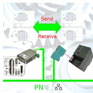
Coupling S7-controller with MPI/Profibus at S5-control with PD-port via network
