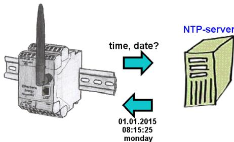
Should all EtherSens devices record time-synchronized in your equipment? By coupling with an NTP-time-server, all devices pick up the current time and adjust this.
