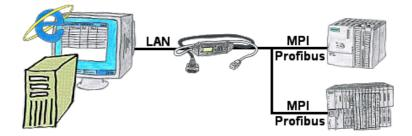
You would like to give your customer the opportunity to read current numbers of the manufacturing Online, without installing a visualisation or even the STEP7-package? Then a S7-LAN with the option Status Variable" is needed, and your customer can take a look at these password protected data on a site of the integrated webserver.
