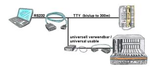
Universally to the S5-PLC, free 9-pin COM-port is sufficient on the PC and free PG-port on the PLC.
