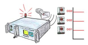
You need some limits? No problem, with the OSC-II-devices you will be able to define 3 relay outputs (toggle switch) like UG (down level) or OG (top level) or as a ready-flag (internal probe has working temperature).
