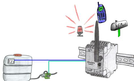
Apply small control tasks of your systems with EtherSens-Control-devices. Determine switching points where the device is running to respond. Depending on the parameterization, an email or SMS notification (depending on the device-configuration) or the device automatically controls via the optional IO-modules (analog / digital / relay).
