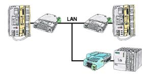
Your pumping stations report the water levels of the central control via telephone network. The central office itself can of course transmit commands/messages to the substations as well. Therefore no dedicated line is required, it's sufficient when the stations connect via network (DSL-router).
