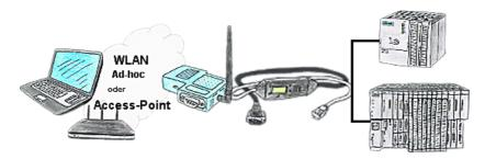
Your're right in the middle of your production line and and should move around the machine and simultaneously observe / manage. No problem, you parameterize the S7-WLAN-Bridge, connect to the MPI-LAN and connect to an access-point or with the ad-hoc-network of your laptop and are ONLINE on the PLC.
