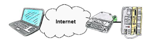
You have access to a on-site network and your PLC has no LAN-connection? No problem, plug the S5-LAN on the PLC and you will have immediate access to the PLC from afar.
