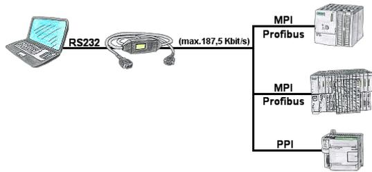
With the MPI/PPI-cable you have the ability to access a connected SPC-PLC S7-200 (PPI 9600 Baud and 19200 Baud) as well as S7-300/400 (MPI/Profibus 9600 Baud up to 187500 Baud) via PC serial with up to 115200 Baud for reading respectively writing of data.
