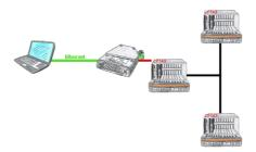
With the S5-H1-PG-LAN you would be able to use the H1-path-selection over the S5-LAN++ and communicate with all PLCs in the H1-bus. You dont have to connect serial to the CP, you can do this easy over your network.
