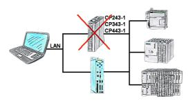
Do you have a PLC without CP343-1 or CP443-1 and a TP-II as remote maintenance device? Then activate the CP-mode of the TP-II and your visualisation goes directly ONLINE via the LAN of the TP-II.
