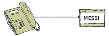
The MESSI remote-station will be called directly by integrated mobile-phone. If a connection comes off, digital In- and Outputs for teleswitching will be transmitted. Each device can both transmit state of things and accordingly receive switch signals.
