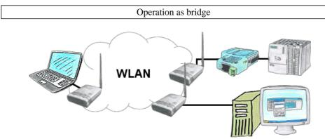
You have two or more clients which should communicate together without LAN-cable-connection? No problem, you connect a "Access-Point" configured ALF to this device and to the other device a "Client" configured ALF. Then connect the "Client" with the "Access-Point" and the device are able to communicate together.
