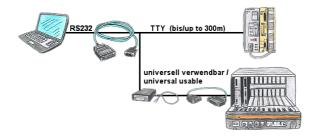
Universally to the S5-PLC, free 9-pin COM-port is sufficient on the PC and free PG-port on the PLC.
