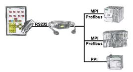
Your panel provides a serial port and no MPI/Profibus for connecting a S7-PLC. Connect the MPI/PPI-cable with it and you're Online with your panel.
