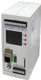
The Messi is a fault-messenger which sends its fault-messages via the GSM-network. As a result, it is not affected by german telekom's switch to the digital telephone-network.
