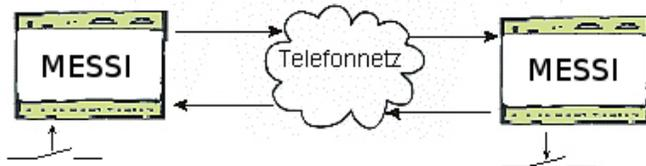
The MESSI will be called by conventional Telephone or by mobile-phone. With a direct voice message and DTMF-tone dialling the corresponding output will be set-up. If a switching operation has come off a speech output will confirm it.
