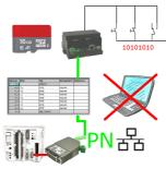
Via digital input triggered DB-backup/-restore without additional PC via PG-socket and Ethernet to SD-card
