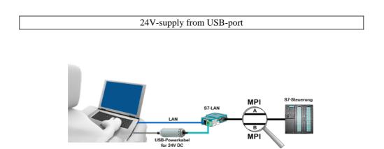
On site at your system, in the middle of the field and no 24V supply for your e.g. S7-LAN-module?
