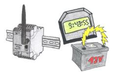
You always need a current time, but do not always have a time-server on site. With the integrated battery-backed RTC you always have the current time in the unit. Even if the power fails, the time in the unit continues to operate, so that when the voltage returns, the time continues to run correctly.
