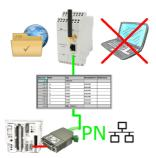
S5-PLC triggered DB-backup/-restore without additional PC via PG-socket and Ethernet on FTP-server
