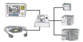
Do you have a single control with panel in use and have to accomplish a little modification in the control program? No problem, plug the T-Connector on the PLC, the panel and PC to the device and then both participants can work with the PLC without annoying bus-cable tapering and interconnections.
