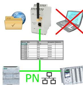
S7-PLC triggered DB-backup/-restore without additional PC via PN-port on FTP-server
