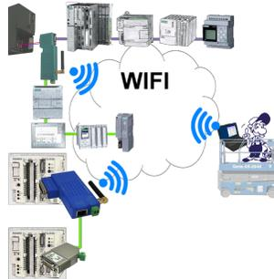
Wired or wireless communication (WIFI) via the same adapter with the respective control Devices from the BRIDGE-family always connect a wired-network with a wireless-network (WIFI) and a specific PLC-interface. This gives you access to the directly connected controller via WIFI (with S7 to the entire bus) as well as to the wired Ethernet. Of course also from wired Ethernet to WIFI and control/bus.
