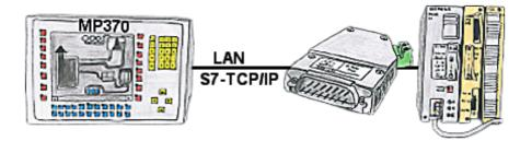
Your panel only has a LAN-socket as PLC-interface and supports only S7-RFC1006, no problem. Connect this socket with the S5-LAN++ and plug it directly on the PD-interface of the PLC. The S5-LAN++ performs adverse your panel as a S7-PLC although you receive the data from the S5-PLC. Then access to the variables and data of the S5-PLC is already available.
