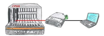
Your visualisation-software does not support a 3964R-protocol, but you have to apply this package? No problem, connect the 3964R-LAN to your CP and activate the RFC1006-emulation in the module. Now your software gets the data from the module via RFC1006, which in turn communicates with the assembly via 3964R.
