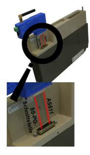
• the system also acts as an S5 network adapter for programming, Remote maintenance and for coupling the different PLC controls
