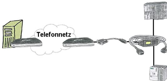
You have to reach urgend your PLC via remote maintenance and have no TS-adaptor in your company? No problem, configure with the MPI-Kabelmanager your S7-interface-cable MPI/PPI-Kabel the mode "TS" for "remote maintenance", connect this cable with the TS-Adapter (article number 9350-TS) with a standard modem and send it all to your client. Now you will be able to start the connection with your TS-software and solve the problem. And this all without buying a original TS-adaptor.
