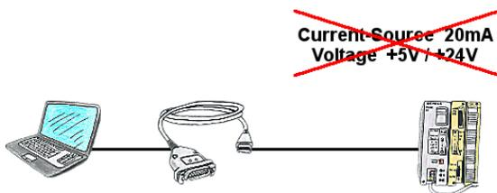
PLC's without current-sources (+20mA) and voltages (5V/24V) at the PG-interface such as the AS511-plug-in card?
