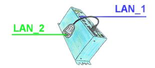
You need a separation between the machine-net and the office-net? No problem, plug a PCMCIA-LAN-card in your Tele-Prof-II-device (only for version -H) and the separation is OK. You have access to both nets via remote maintenance.
