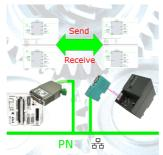
Coupling S7-controller with MPI/Profibus at S5-control with PD-port via network
