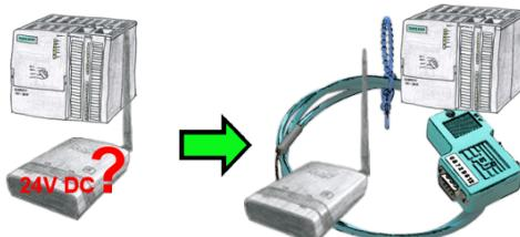
You want to install your ALF directly in the switch-board and would like to use the 24V of the existing S7-PLC? No problem, connect the open ended side of the Kabelbrücke to the 24V port on your ALF and the bus-side on the MPI- or Profibus of this PLC. Even the ALF is supplied above this PLC.
