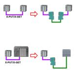
MPI/DP communication between two S7-300/400 controllers on the same bus - a control is relocated spatially:
